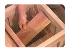
The planter box was designed so that the height of the bottom could be easily adjusted to suit Donna's needs. Using blocks of 2 x 6s or 2 x 4s, depending on the height they wanted, they laid the blocks up against the insides of the box and then set planks across the blocks to create the bottom.
