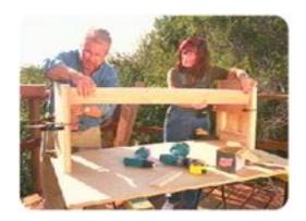
After completing the two end panels, Ron used clamps to position the end panels to stand up on their own, which would make it easier for them to complete the assembly. Ron also clamped in place a temporary ledger onto each end panel that would help them hold the first stretcher in place while they attached it. The stretcher would connect the two end panels together.
