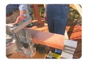
Ron set up an adjustable stop block on the saw. Since they would be cutting sixteen pieces of lumber to the same length, the stop block would ensure consistently accurate cuts. After a quick lesson on the power miter saw, Donna was comfortable cutting all the lumber.
