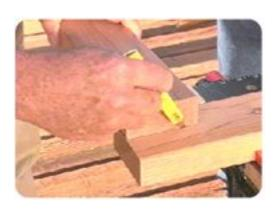
He showed Jennifer how to push this template up against the piece of wood that was to be notched. When the block touched the edge of the wood, he traced the outline right onto the piece to be cut.
