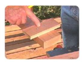
Ron measured and determined the size of his notch and then created a template by nailing a small piece of wood to a larger piece.
